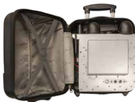
Special, camouflaged portable execution of PIK-GAT, dedicated for foot patrols and teams not provided with built-in vehicle gateway
