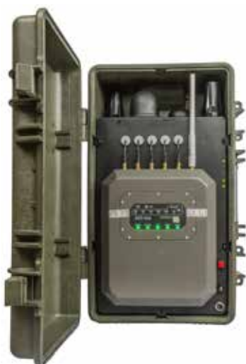
Special, rugged portable execution of PIK-GAT, dedicated for foot patrols and teams not provided with built-in vehicle gateway
